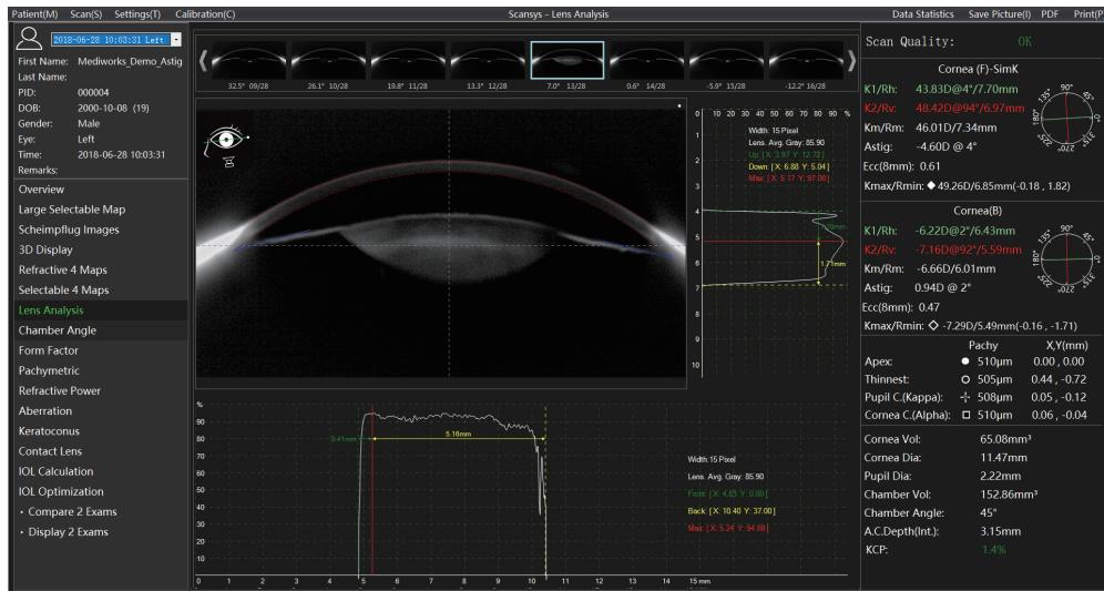
Scansys calculates the lens density value for cross section and longitudinal section which is helpful in cataract diagnosis.
