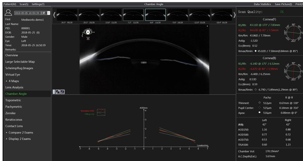
Scansys can calculate a chamber angle value based on the tomography images and its exclusive AOD graph gives a trend analysis for the distance between cornea back surface to iris. It also provides cornea volume, anterior chamber volume and anterior chamber depth calculation. These analyses is helpful to glaucoma diagnosis.
