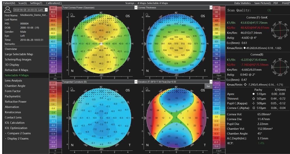
Click on the “Selectable 4 Maps” to open a window contains 4 optional color maps. Corneal thickness and elevation, etc. can be loaded into one of any 4 fields.
