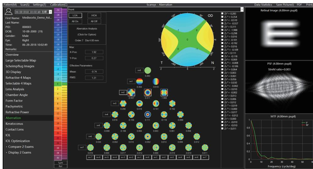
This view is a Zernike analysis of the measured corneal front, back and all surface height data, which calculates a factor for each Zernike polynomial term that describes the contribution of this polynomial to the height data. To guide the visual quality analysis of refractive surgery.
