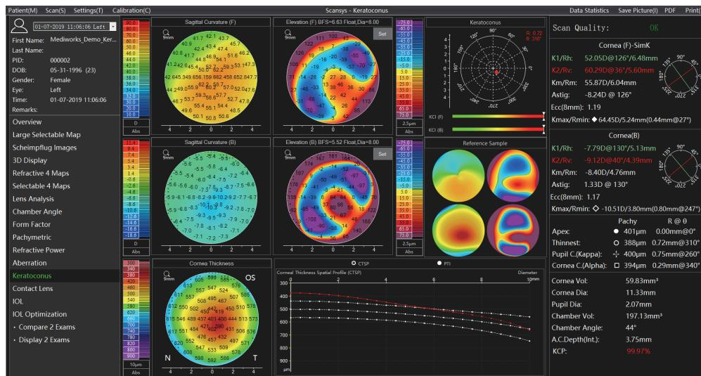
Scansys introduces AI algorithms to more intelligently give the possibility of Keratoconus (KCP) ( Reference value: KCP, range 0% –100% ) The above figures contain the topographic maps of Refractive 4 Maps, and the axial curvature map of the back surface, and the trend distribution of the thickness map is also given. These are the key references for judging the keratoconus.
